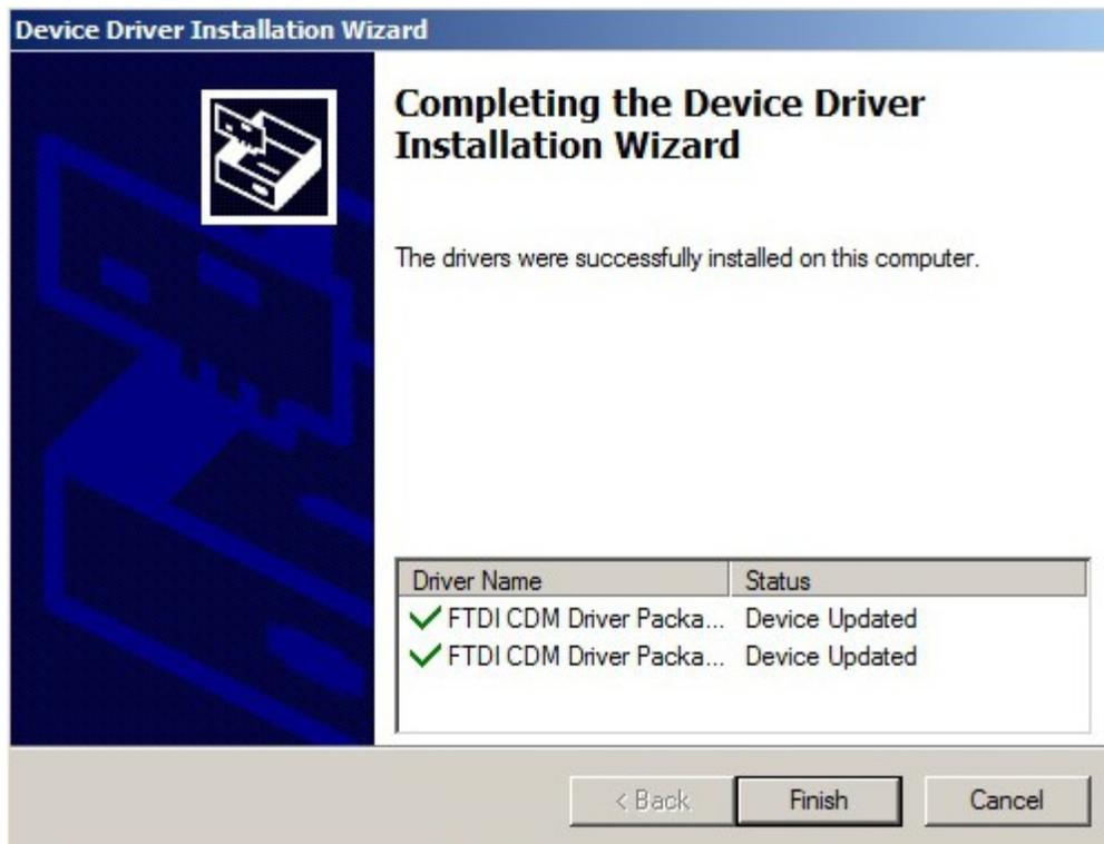
Now plug in the Lean Protection Module if you haven't already and your PC will detect it and assign it a COM port. To find out which COM port it assigned go into Control Panel. From there we will select "Device Manager"
